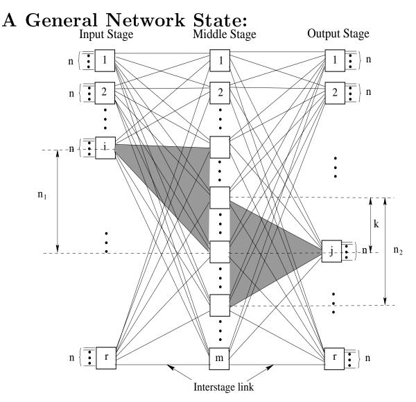
A three-stage Clos network with  $n_1$  busy input-middle interstage links from input stage switch i,  $n_2$  busy middle-output interstage links to output stage switch j, and k pairs of the interstage links overlapped.
