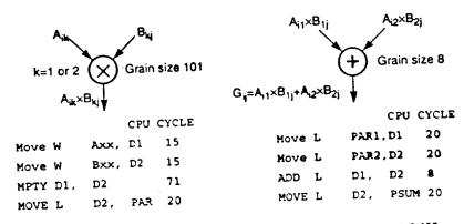
(a) Grain size calculation in M68000 assembly code at 20-MHz cycle
