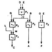
(b) Sequential execution in five steps, assuming one step per statement (no pipelining) (c) Parallel execution in three steps, assuming two adders are available per step
