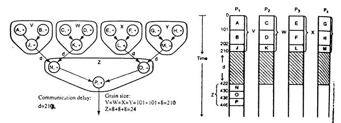
(a) Grain packing of 15 small nodes into 5 bigger nodes (b) Parallel schedule for the packed progra
