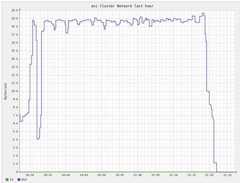
Figure 18: Throughput achieved by RFTP in the ANI testbed 100Gbps network.
