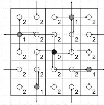
Fig. 1. Circuit-switched and wormhole routing mesh network
