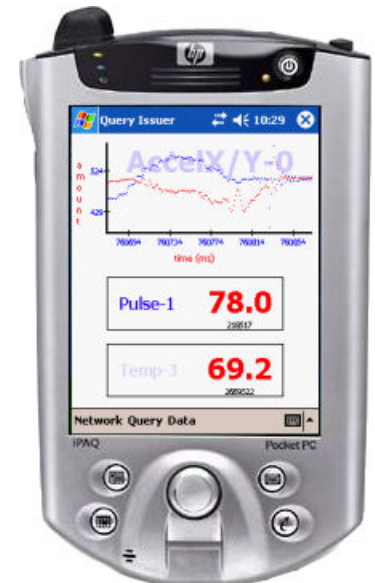
Figure 4: A GUI displays accelerometer data, patient pulse-rate, and environmental temperature.
