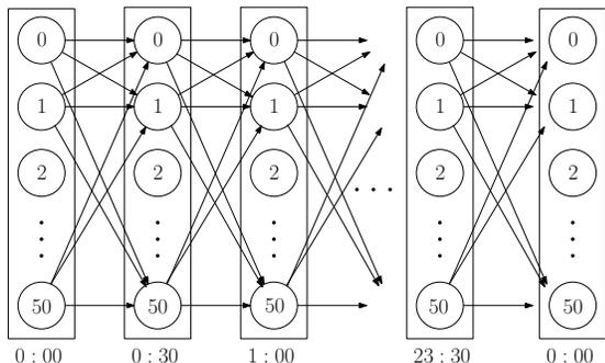
**Fig. 2: Occupancy dynamics as Time Inhomogeneous Markov Chain unrolled for one day**
