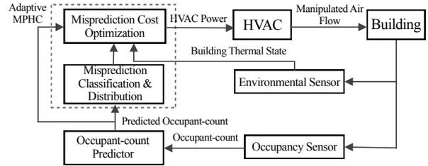
Fig. 9: Adaptive Model Predictive HVAC Control Architecture
