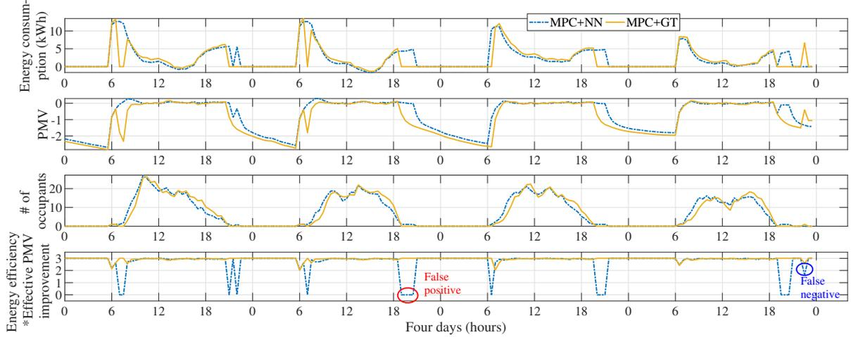
Fig. 8: Performance of MPHC using predicted occupant-count (neural network) and ground truth over 4 days
