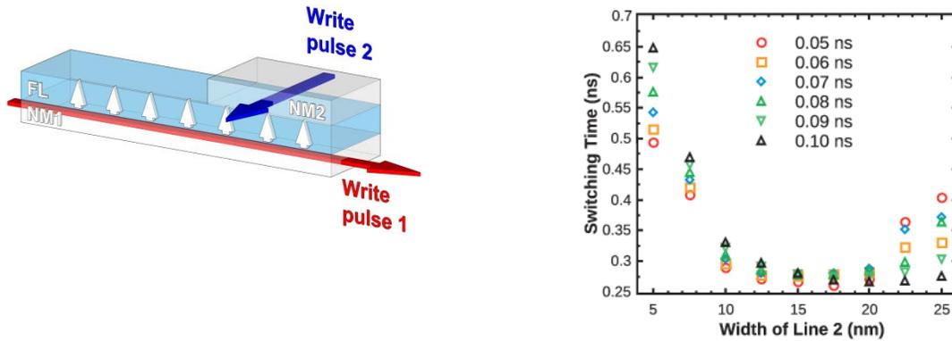
Fig. 1. (a) Perpendicular SOT-MRAM memory cell with a 52.5x12.5x2 nm free layer; (b) Switching time vs. line 2 width, for several durations of the pulse 2,  $I_1 = I_2 = 100 \mu\text{A}$ .
