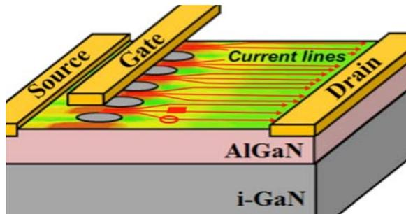
Fig. 2. Two-dimensional simulation of a perforated channel [G. S. Simin *et al.*, *IEEE EDL* **35**, 449 (2014)].
