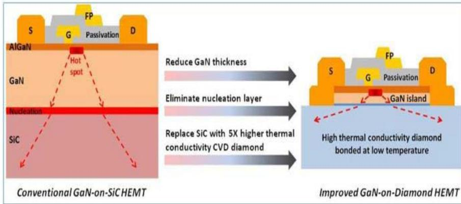
Fig. 1. Heat removal by diamond [P.-C. Chao *et al.*, *IEEE TED* **62**, 3658 (2015)].
