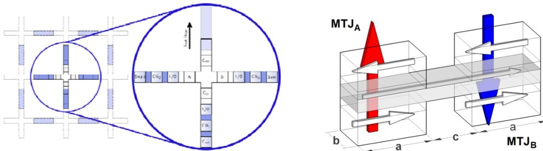
Fig. 1. (a) Spin torque majority gates (crosses) perform the computation, while the nonvolatile flip-flops (rectangles) act as shared buffers. A single STMG and three flip-flops are sufficient to realize a concatenated 1-bit full adder; (b) Schematic illustration of a spin-torque oscillator based on two MTJs. The colored arrows indicate the direction of the current for each of the MTJs.
