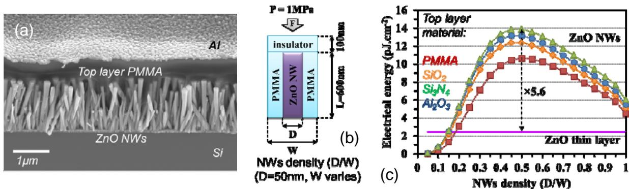
Fig. 1: VING structure and performances under compression. (a) SEM Image of a VING built on silicon, with ZnO NWs embedded in PMMA; (b) side view of a VING elementary cell, where D is the NW diameter and W is the cell width; (c) simulated energy generated by a VING cell in mechanical compression [7].
