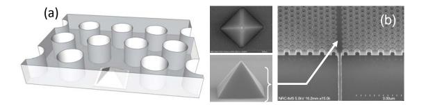
Fig. 1. (a) Schematic illustration showing the alignment of a single, site controlled InAs/InP quantum dot to the defect site of a membrane microcavity. (b) SEM images of a single dot waveguide device at various stages of fabrication.
