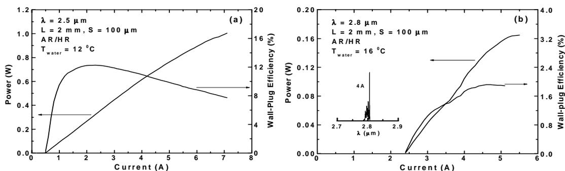
FIG. 1: Continuous wave operation of 2.5  $\mu\text{m}$  (a) and 2.8  $\mu\text{m}$  (b) GaSb-based lasers.
