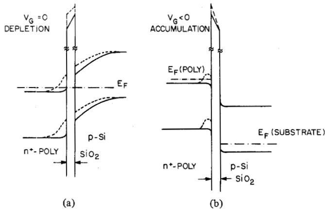
Fig. 2. Band-diagrams of the polysilicon-oxide-silicon gate structure. (a) Depletion or weak inversion at  $V_G = 0$ . (b) Accumulation,  $V_G < 0$ . For clarity, the pictures are drawn with different scales in polysilicon (where the depletion depth is of order 100 Å or less) and Si (where this depth is  $\leq 1 \mu\text{m}$ ).
