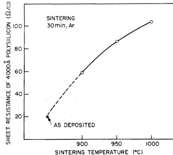
Fig. 3. Sheet resistance of 4000-Å polysilicon film after 30-min sintering with a tantalum silicide cap. The increase in resistivity is associated with the depletion of phosphorus caused by its diffusion into the silicide.
