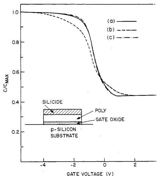
Fig. 1.  $C$ - $V$  characteristics of MOS capacitor with silicide gates; (a) before sintering; (b) after 30-min sintering at  $900^{\circ}\text{C}$ ; (c) after subsequent phosphorus diffusion (15 min,  $900^{\circ}\text{C}$ ) with silicide layer removed.
