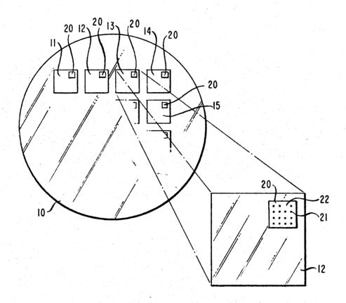
For many purposes, especially device development, production and quality control, it is important to know the originating location of a semiconductor chip on a wafer. It is desirable that means for so identifying chips be machine readable as well as visually readable, and that such chip identification require a minimum quantity of data for its specification.
