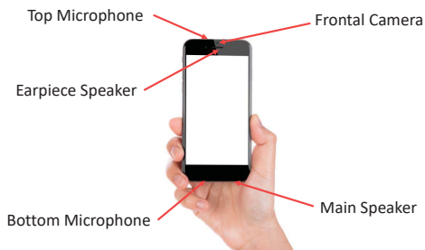
Figure 3: Typical layout of speakers, microphones and camera on smartphones.
