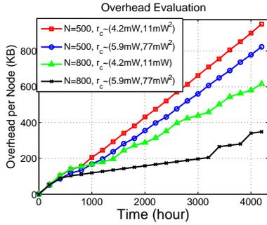
Fig. 7. Average overhead for each sensor node per second.
