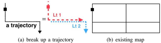
Fig. 3. (a) break up a trajectory sample into multiple L-components ( $L_t$ ). (b) existing map can also break into multiple L-components ( $L_m$ ) and then match with  $L_t$ . A square represents a speed bump detected.
