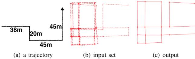
Fig. 1. (a) a trajectory represented as:  $0^\circ, 38, -90^\circ, 20, 90^\circ, 45, 90^\circ, 45$ . (b) and (c): the input set is 10 trajectory samples from a parking lot, and the output is the reconstructed map.
