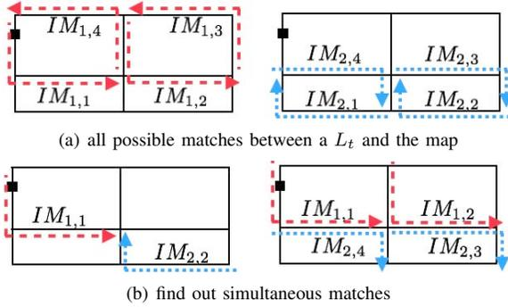
Fig. 4. (a)  $L_t$  can independently match to the map in 4 ways, so is  $L_t$ . (b)  $IM_{1,1}$  and  $IM_{2,2}$ , for instance, cannot happen simultaneously, otherwise the geometrical shape of the trajectory will be unable to maintain. Finally, only two combinations are left:  $(IM_{1,1}, IM_{2,4})$  and  $(IM_{1,2}, IM_{2,3})$ .
