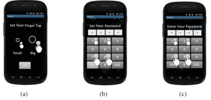
Fig. 1. Screenshots of TapLock as a 4-digit PIN system. (a) Setup of a finger tap’s label: The finger tap matching the small (or big) circle is automatically assigned a small (or big) tap label. (b) Setup of a TapLock password: The big (or small) finger icon shows a big (or small) touch area. The icons in the figure are for illustration purposes, which are not visible to users. (c) Enter password on a keypad with a fixed layout.
