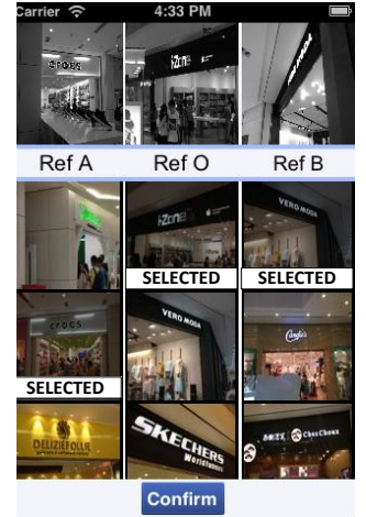
Fig. 2. The UI presented to the user for correction of image matching results. The top row are the 3 test images taken by the user, below each are the top 3 matched reference points.
