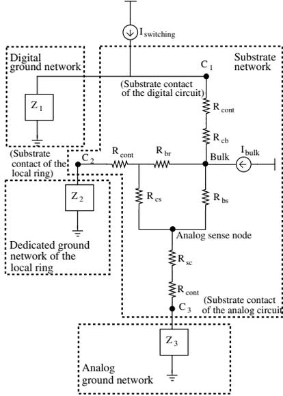
Fig. 5. Equivalent circuit model to analyze the effect of the localized guard ring consisting of the ground network of the digital circuit ( $Z_1$ ), ground network of the local guard ring ( $Z_2$ ), and ground network of the analog circuit ( $Z_3$ ). The substrate network is represented by the equivalent resistance among the substrate contacts and the analog sense node.
