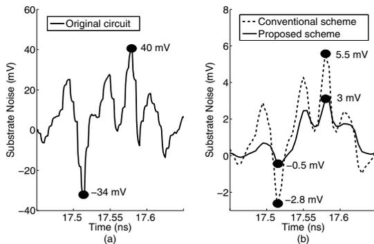
Fig. 8. Substrate noise voltages observed at sense node 2: (a) The original circuit, (b) Conventional and proposed guard ring schemes.
