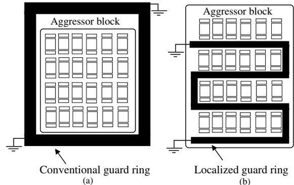
Fig. 1. Simplified representations of (a) conventional guard ring around an aggressor block, (b) proposed localized guard ring within an aggressor block.
