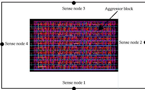
Fig. 7. Layout of the aggressor digital core located close to a sensitive block in an industrial transceiver circuit. The substrate noise is observed at the four sense nodes located on each side of the block.
