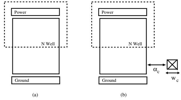
Fig. 3. Standard cell: (a) Conventional cell, (b) Noise aware cell with a dedicated substrate contact for the local guard ring.  $\alpha_c$  is the minimum distance between the contact and the diffusion, and  $w_c$  is the width of the contact.
