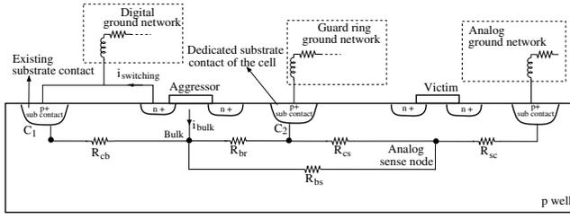
Fig. 4. The effect of the local guard ring on reducing substrate noise. The noise injected from the noisy contact  $C_1$  and bulk of the aggressor device is filtered through the dedicated contact  $C_2$  of the guard ring rather than propagated into the substrate.
