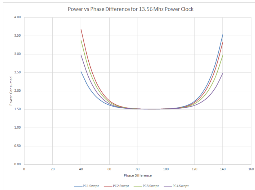
FIGURE 4.6: Overall power consumption in \mu\text{W} (summation of the power consumed by each power-clock signal) vs. phase difference (in ^\circ ) for 13.56 MHz power-clock frequency when only the phase difference of one power-clock signal varies (with respect to the following power-clock signal).
