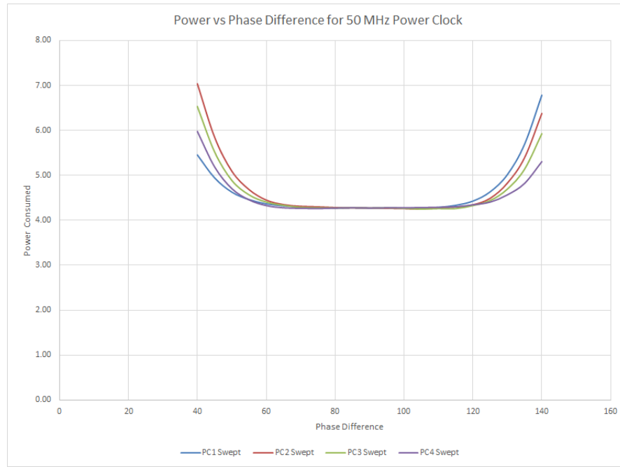
FIGURE 4.7: Overall power consumption in \mu\text{W} (summation of the power consumed by each power-clock signal) vs. phase difference (in ^\circ ) for 50 MHz power-clock frequency when only the phase difference of one power-clock signal varies (with respect to the following power-clock signal).
