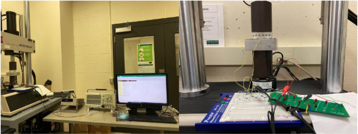
Figure 4.6: Experimental setup to test the PCB prototype of the enhanced frontend electronic circuit with the triboelectric harvester.
