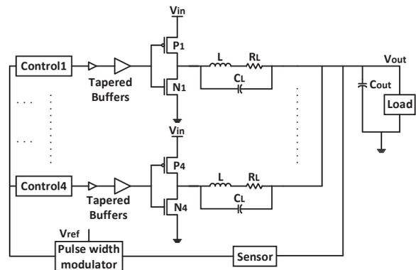
Fig. 1: Interleaved multi-phase switching buck regulator topology.
