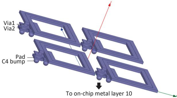
Fig. 4: Array of package-embedded spiral inductors modeled in full wave electromagnetic simulator HFSS.
