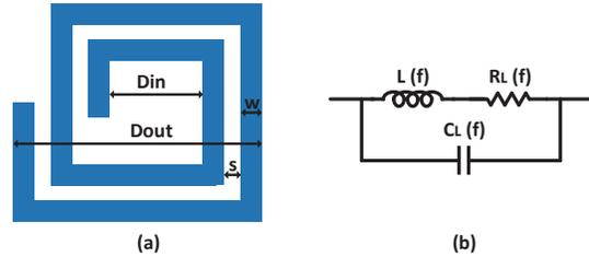
Fig. 3: Typical spiral inductor: (a) physical characteristics, (b) equivalent electrical circuit.
