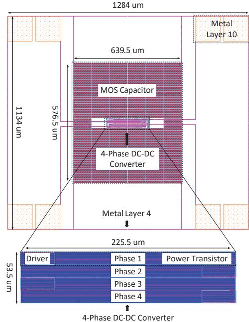
Fig. 6: The on-chip layout of the 4-phase converter, illustrating the power transistors, drivers, MOS capacitors, and metal layer 10 for connection to the package-embedded inductors.
