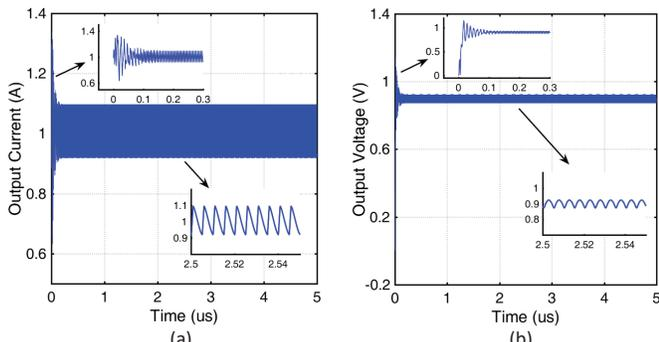
Fig. 8: Simulation results of the interleaved, four-phase buck converter with package-embedded spiral inductors: (a) output current, (b) output voltage.
