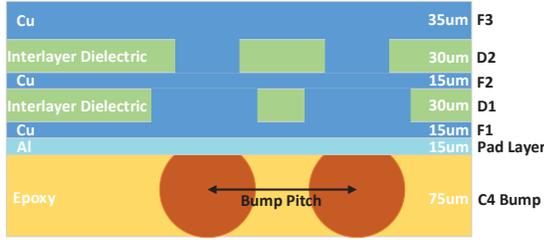
Fig. 2: Cross-section of the multi-layer flip-chip package where spiral inductors are built.
