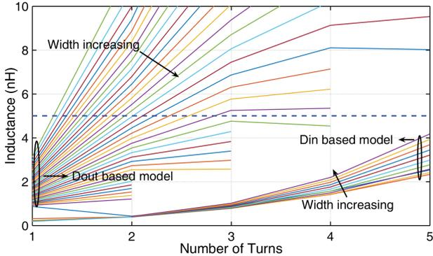
Fig. 5: Design space of the package-embedded spiral inductor as a function of number of turns and width at constant spacing, thickness, and frequency.
