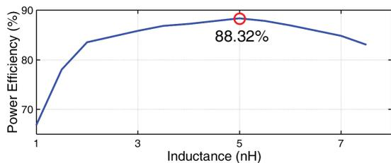
Fig. 7: Power efficiency of an interleaved four-phase buck converter as a function of inductance.
