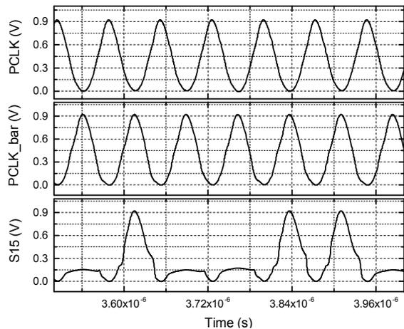
Fig. 6. Simulated voltage waveforms for the 16<sup>th</sup> bit of the adder and the two out-of-phase AC power signals after the signal shaper.
