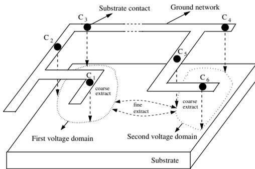
**Figure 1: Identifying the voltage domains within the substrate. Assuming  $V_{C1} \approx V_{C2} \approx V_{C3}$  and  $V_{C4} \approx V_{C5} \approx V_{C6}$ , two voltage domains are created by the first and last three contacts. A coarse extraction is performed within each domain to reduce the computational complexity, followed by a fine extraction of those domains where the dominant current flow occurs.**
