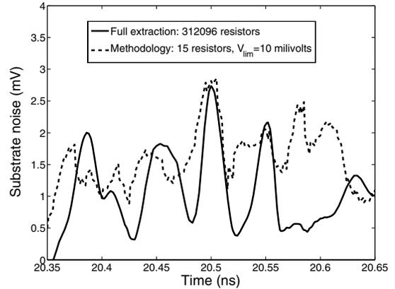
**Figure 9:** Comparison of the substrate noise at the sense node obtained by simulating the fully extracted circuit and application of the methodology when  $V_{lim} = 10$  mV.
