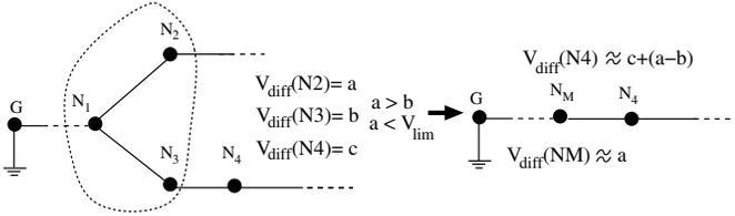
**Figure 5: Illustration of the *Correct* function. After the nodes  $N_1$ ,  $N_2$ , and  $N_3$  are merged based on  $V_{diff}(N_2)$ ,  $V_{diff}(N_4)$  shifts by  $a - b$  which is compensated by the *Correct* function.**
