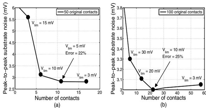
**Figure 10: The variation of the peak-to-peak noise with respect to the number of contacts after merging: (a) The simulation circuit with 50 original contacts. (b) An extension of the circuit with 100 original contacts.**
