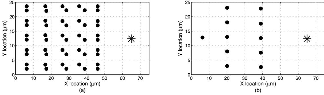
**Figure 4: Physical location of the substrate contacts (represented by the circles) and the sense node (represented by the star) where the substrate noise is observed: (a) original 50 contacts before merging (b) eleven equivalent contacts after merging when  $V_{lim} = 5$  mV.**
