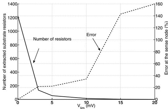
**Figure 8:** Number of extracted substrate resistors and the error in the peak-to-peak noise voltage at the sense node as a function of  $V_{lim}$ .
