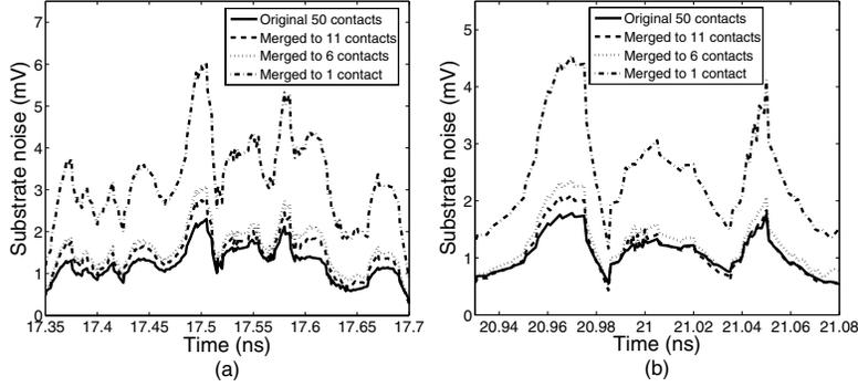
**Figure 7:** Comparison of the substrate noise at the sense node before and after merging for two different time intervals: (a) from 17.35 ns to 17.70 ns (b) from 20.93 ns to 21.08 ns.
