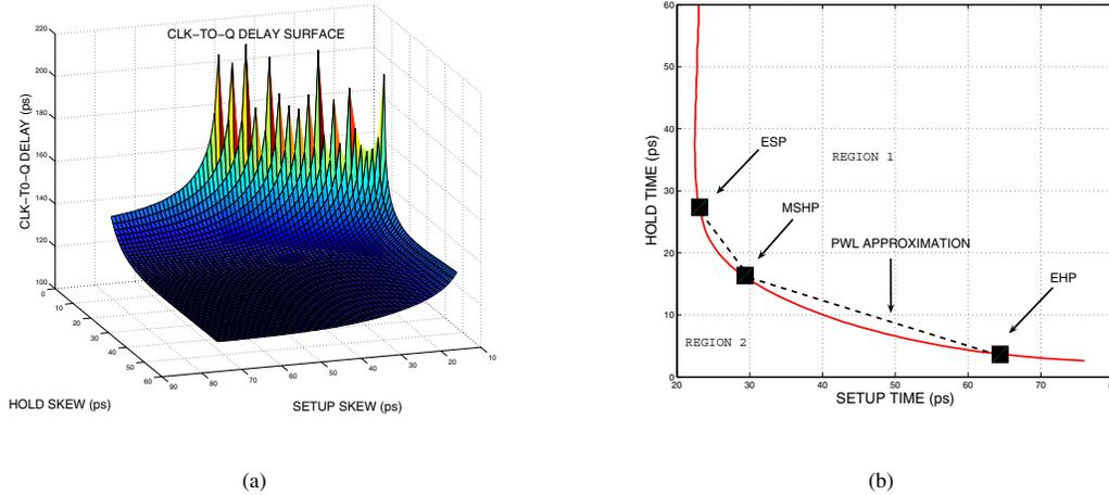
Fig. 4. Interdependent constraint characterization: (a) CLK-to-Q delay surface as a function of independently varying setup skew and hold skew, (b) The contour at 10% degraded CLK-to-Q delay. The contour includes the critical pairs as well as a piecewise linear approximation. Regions 1 and 2 are the pessimistic and optimistic regions, respectively.
