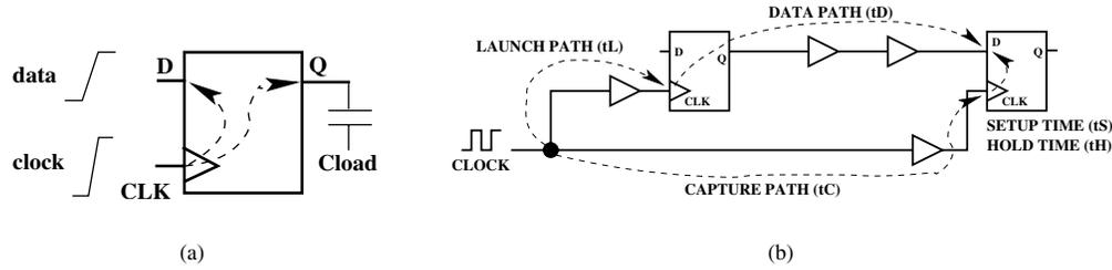
Fig. 1. Register with a synchronous circuit: (a) simplified register, (b) conceptual computation of setup and hold slack in STA on an example synchronous data path.
