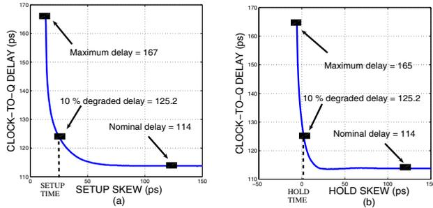
Fig. 2. Independent constraint characterization for sequential circuits: (a) setup skew vs. CLK-to-Q delay for setup time characterization, (b) hold skew vs. CLK-to-Q delay for hold time characterization.
