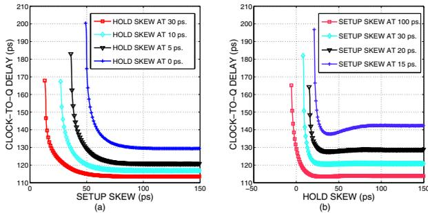
Fig. 3. Constraint characterization for sequential circuits at different counterpart skews: (a) setup skew vs. CLK-to-Q delay at different hold skews, (b) hold skew vs. CLK-to-Q delay at different setup skews.
