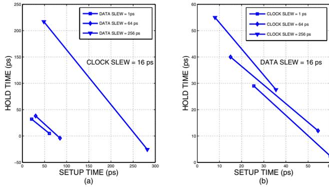
Fig. 6. Linear representations using two pairs, ESP and EHP: (a) at different data slews, (b) at different clock slews.
