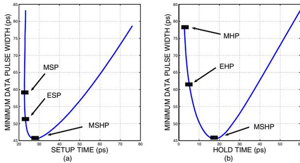
Fig. 5. The relationship between constraints and the minimum pulse width: (a) setup skew vs. minimum pulse width, (b) hold skew vs. minimum pulse width.
