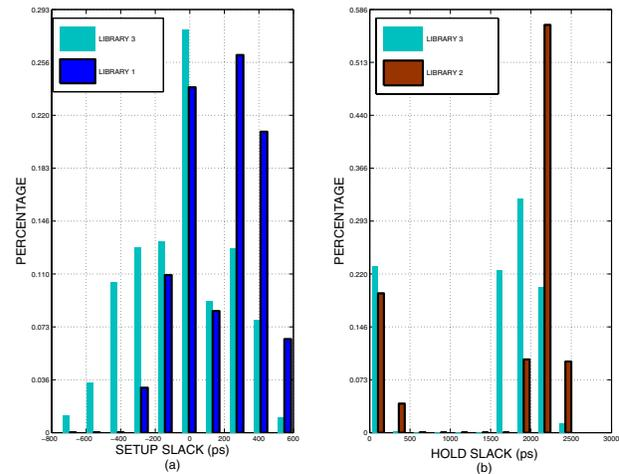
Fig. 10. Slack histograms for circuit B: (a) setup slack histograms of library 3 and library 1, (b) hold slack histograms of library 3 and library 2.
