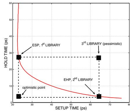
Fig. 8. Constant delay contour curve illustrating the characterization points of the three prototype libraries.
