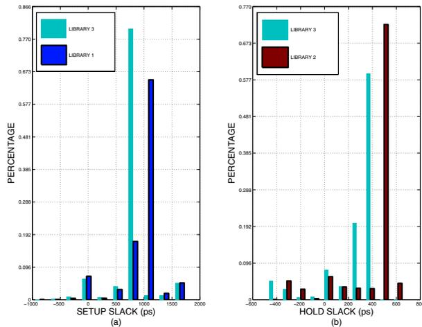
Fig. 9. Slack histograms for circuit A: (a) setup slack histograms of library 3 and library 1, (b) hold slack histograms of library 3 and library 2.
