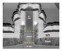
FIG. 1. Cross-sectional SEM image of the GaN-based vertical nanowire transistor.
