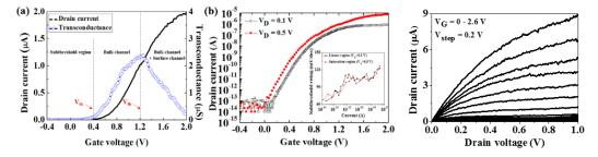
Fig. 2. Transfer (left) and output (right) characteristics of device.
