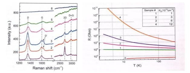
Fig. 1. Raman scattering vs.  $C^+$  ion irradiation (left); temperature dependence of irradiated films vs. defect density  $N_D$  (right).
